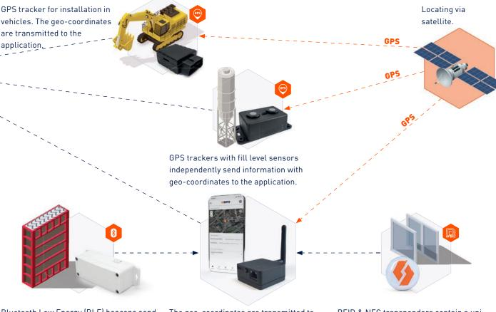
Bluetooth Low Energy (BLE) beacons send their signals to a BLE hub or a smartphone. The geo-coordinates are transmitted to the application via smartphones or BLE hubs with connection via WLAN, Power over Ethernet (PoE) or an LTE-M card. RFID & NFC transponders contain a unique identification number that can be read by certain readers or smartphones.
