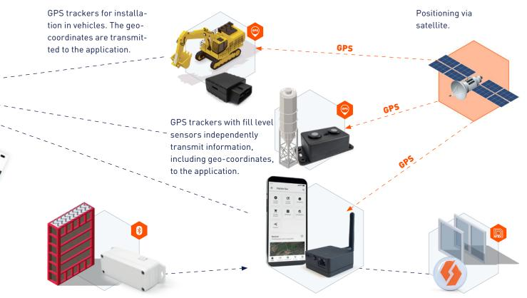
Bluetooth Low Energy (BLE) beacons transmit their signals to a BLE gateway or a smartphone.
